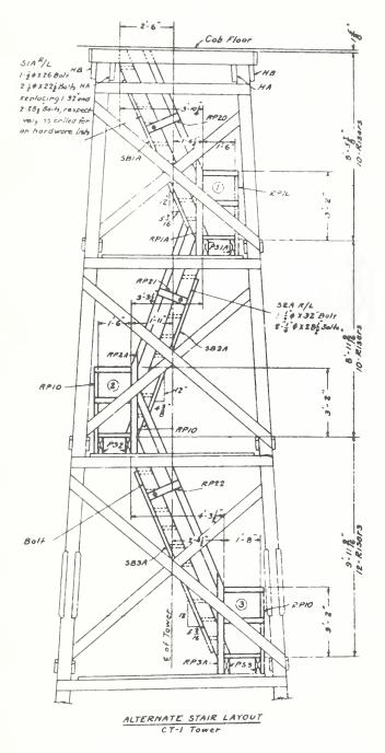
Figure 65. This figure reproduces a small section of a plan entitled "Alternate Details: Standard Lookout Tower Type CT1, for 52, 66, 82, 99 and 119 ft. Heights." This design was for use with 7 feet square tower cabs which did not have a catwalk. This particuar plan was drafted in Region 6 (Pacific Northwest) under the direction of James Frankland, Regional Engineer. Compare this design with Figure 63.
